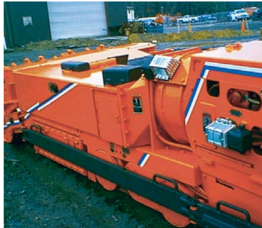
Englo Type 27 Mounted on Joy 14cm15 Continuous Miner-Over 18,000 cfm
